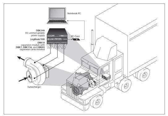
Monitoring key parameters in and around the turbocharger allows engineers to assess the performance of the design.
